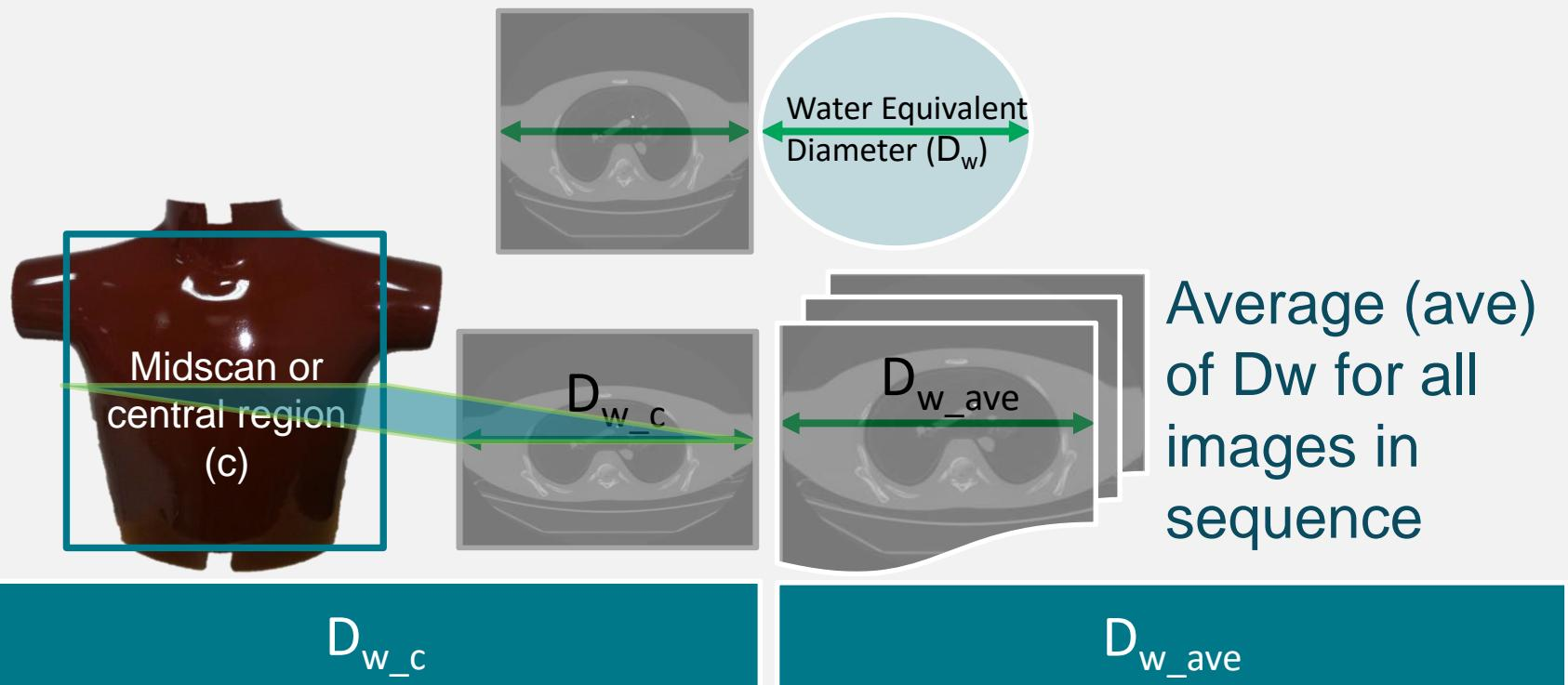
SSDE calculated using  $CTDI_{vol}$  and  $D_{w\_c}$ , according to definition
